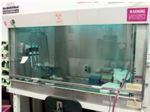
Biosafety cabinet. Source: LBNL EH&S
